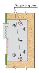
4 Insertion of the male part + fixing through screws and pins.
