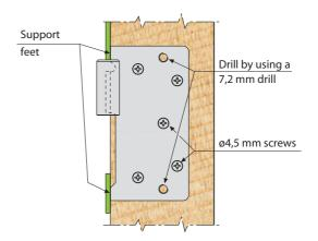
3 Drilling + fixing supporting pins.
