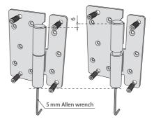
**ADJUSTABLE:** in height thanks to the Allen head screw placed on the base of the hinge body which make it possible to vary the height up to 6 mm.
