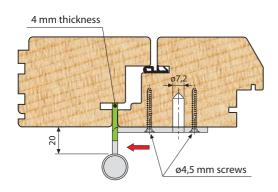
2 Fixing by using ø4,5 mm screws
