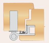
For profiles with gasket on rebate, 10/12 mm
