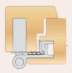
For profiles with gasket on rebate, 15/18 mm
