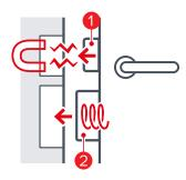
The magnetic movement latch creates new silence standard when the door closes.
