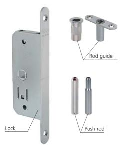
The forend does not have any spring latch, bolt or hook and is completely smooth. The door is closed by means of a push rod mounted on a threaded bar with 30 mm travel which is operated by a 180° follower rotation.
